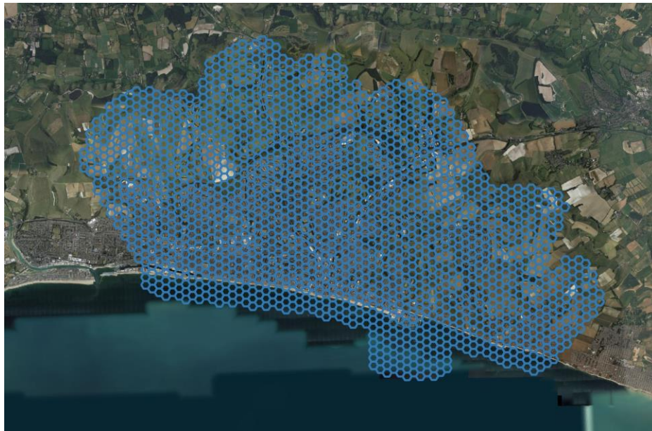
Figure 1: Brighton AOI, showing the 300m hex grid across which UHI is analysed.
